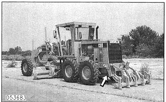
D53683 Inspect the cooling system for leaks, faulty hoses and trash buildup. Correct any leaks and remove any trash from the radiator.
