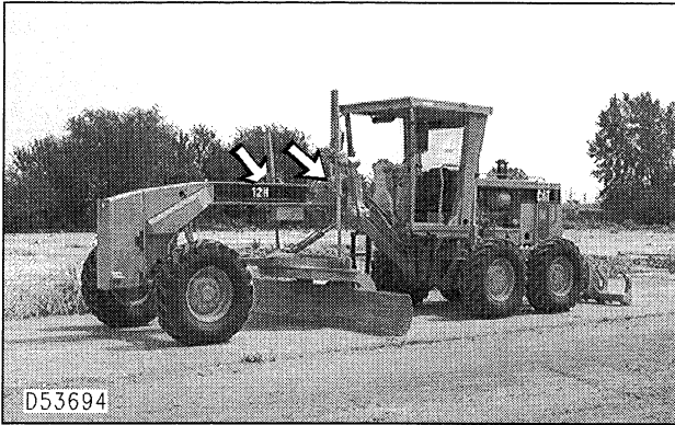
D53694 Inspect the blade linkage for damage, loose or missing bolts. Repair if necessary.
