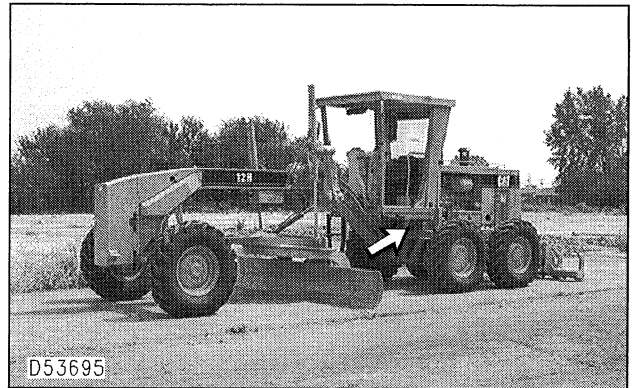
D53695 Inspect and remove dirt and trash buildup in the articulation area.
