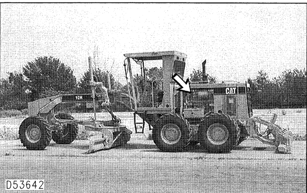
D53642 Inspect and remove any trash buildup in the engine compartment.
